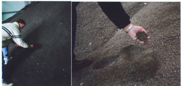
Treated stockpiles remain loose and easily workable. The materials do not break down, clump or harden. This pile was treated in August 2008, the photos were taken in late March 2009.
